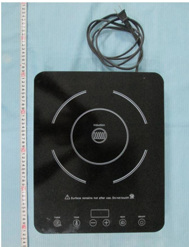
Figure 2: A photo of a single-burner induction range taken at a testing facility (Bay Area Compliance Labs Corp 2015)
