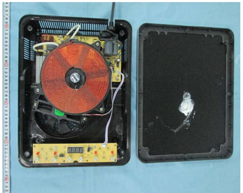
Figure 1: Single-burner induction range with its faceplate removed showing internal components; the copper coil (center) produces the magnetic fields which heat cookware (Bay Area Compliance Labs Corp 2015)
