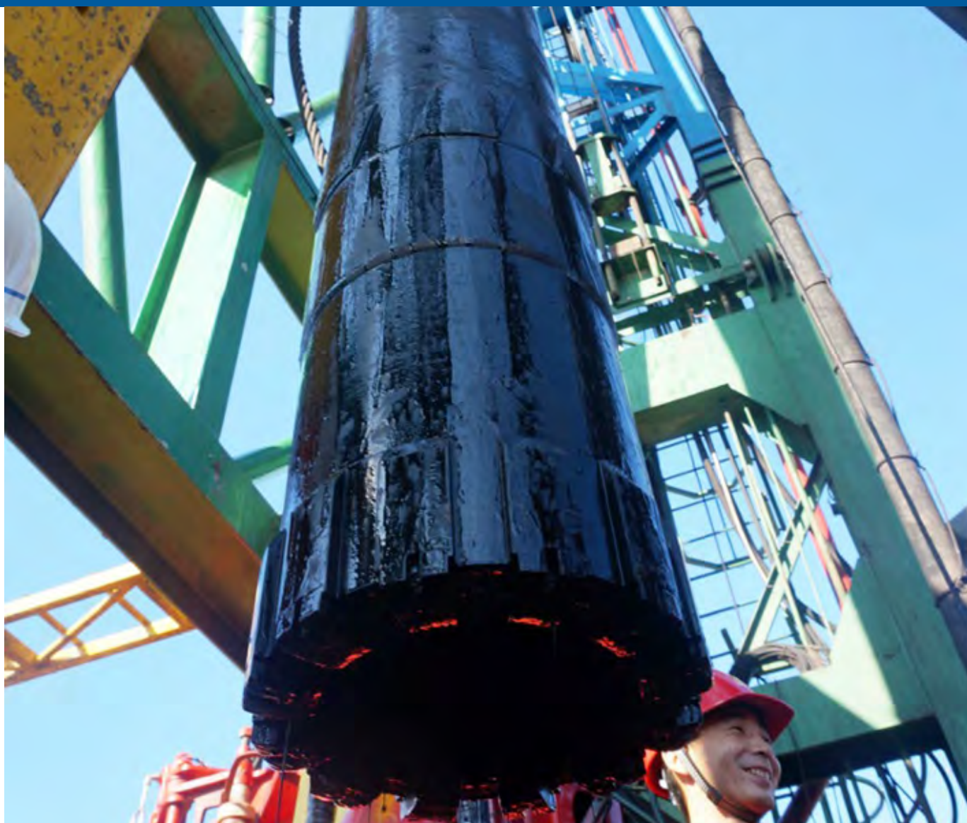
The Continental Scientific Drilling Project of Cretaceous Songliao Basin (SBDP) reached 7018 m depth with a newly designed drill rig and recovered up to 40 m long cores of more than 20 cm diameter. The core samples allow the unravelling of the climate and environmental evolution of the entire Cretaceous period.
