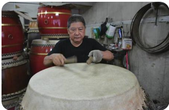
▲繃鼓製程鼓棒敲打鼓面測試
