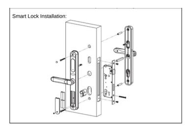
a. Start by removing your current lock. This is generally done by unscrewing the bolts and pulling out your current door knob.
