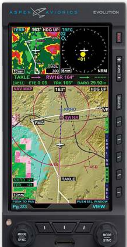
Pantalla ASPEN 500 MFD (MULTI-FUNCTION DISPLAY)
