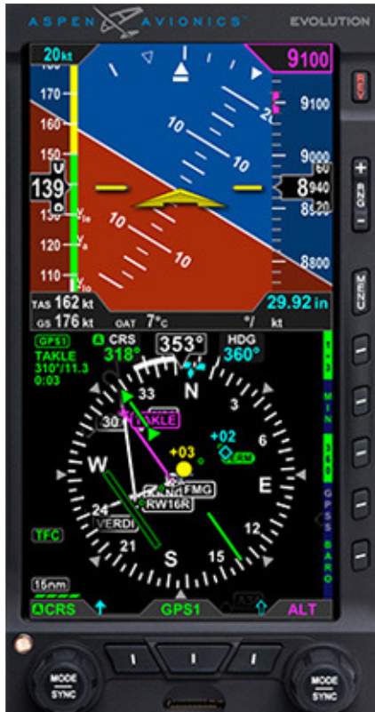
Pantalla ASPEN 1000 PFD (PRIMARY FLIGHT DISPLAY)
