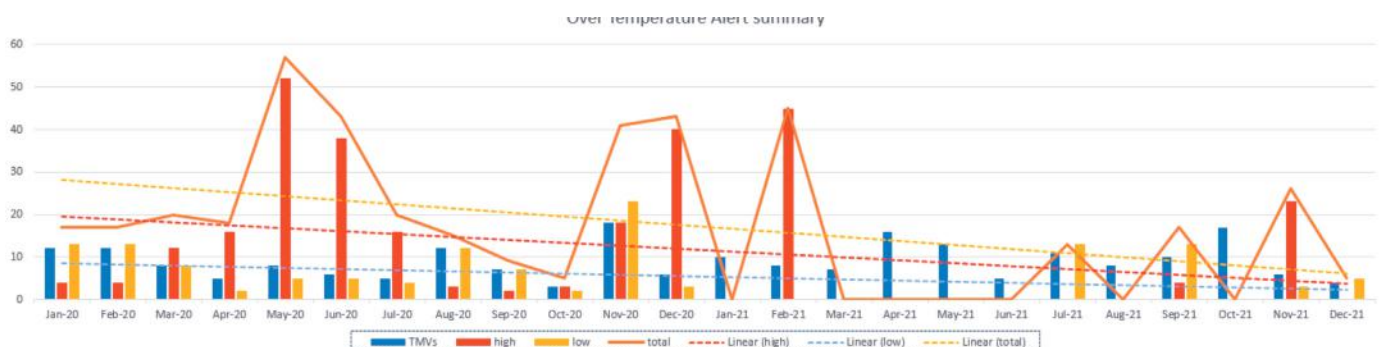
Graph2 – shows significant reduction in over temp alerts (high/low and no# valves) for a 2 year period reducing unplanned maintenance tasks
