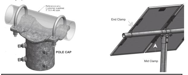
User supplies 4" schedule 40 steel pipe(s) for vertical pole and a 3" schedule 40 steel pipe for the horizontal beam. Calculation of the required horizontal beam length (L) in inches:  $L = 5 + (Q \times W) + ((Q-1) \times 1.28)$  where Q = module quantity, W = module width
