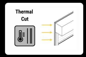
The plastic profiles between the door frame and the fixing wall create a thermal break.
