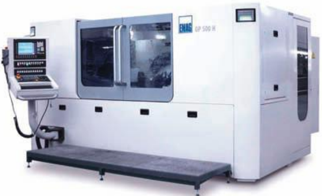
The EMAG GP 500 H was developed for the precision grinding of internal and external gears. For aerospace, helicopter and general gear manufacturing, it guarantees the highest quality, especially for components that have many interfering contours due to their design. The compact design and 5-axis technology guarantee precise results.
