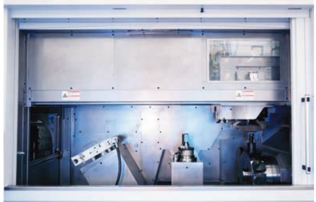
View into the work area of the VLC 350 GT. The machine combines turning, milling and grinding in a single setup and guarantees maximum shape and dimensional accuracy for complex workpieces.
