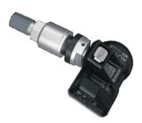
The 1-Sensor is a programmable universal TPMS sensor. It features a combined frequency of 315MHz and 433MHz with aluminum valve stems. The press release button allows for rubber or metal valve stems to be replaced interchangeably. The 1-Sensor is reprogrammable, 99% compatible with OE sensors, and meets SAE standards J1205 and J1206.
