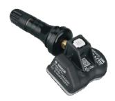
The 1-Sensor is a programmable universal TPMS sensor. It features a combined frequency of 315MHz and 433MHz with rubber valve stems. The press release button allows for rubber or metal valve stems to be replaced interchangeably. The 1-Sensor is reprogrammable, 99% compatible with OE sensors, and meets SAE standards J1205 and J1206.
