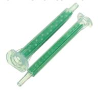
Mix Nozzle for 50 mL, 2:1 or 1:1 dual cartridges. Has 16 elements, a 3.25" length and 5.3 mm inner diameter.
