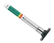
The tire tread gauge calibrated from 0 to 1 inch, reads in 32nds, and three color zones. Red range on bar: 0-3/32nds; Yellow Range on bar: 3/32 - 6/32nds; Green Range on bar: 6/32-32/32nds, which provides accurate depth readings and allows for a quick and easy reading
