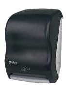
Allows for easy but also extremely sanitary dispensing as users do not have to touch any part of the dispenser to get their towels. Can be set in two operating modes, sensor and towel out. Sensor mode waits for a hand to be placed underneath before it dispenses paper. In towel out mode paper is always available and there is no wait between dispensing. Adjust your paper length as needed (8", 12", 16"). Stub roll feature- automatic transfer system eliminates stub roll waste.
