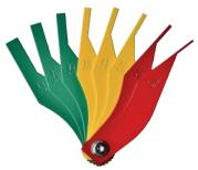
Set of 8 gauges denoting 3 thickness levels: Green, Yellow & Red, which indentify if the brakes are still good (Green), should be serviced (Yellow) and must be serviced (Red)
