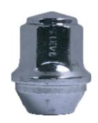
The Chrome Lug Nuts have M14x1.5 Thread Size, 13/16" (21mm) Hex, 1.4" (35.56mm) Overall Length, 0.91" (23.11mm) Width, 60-Degree Conical Acorn /Cone Seat
