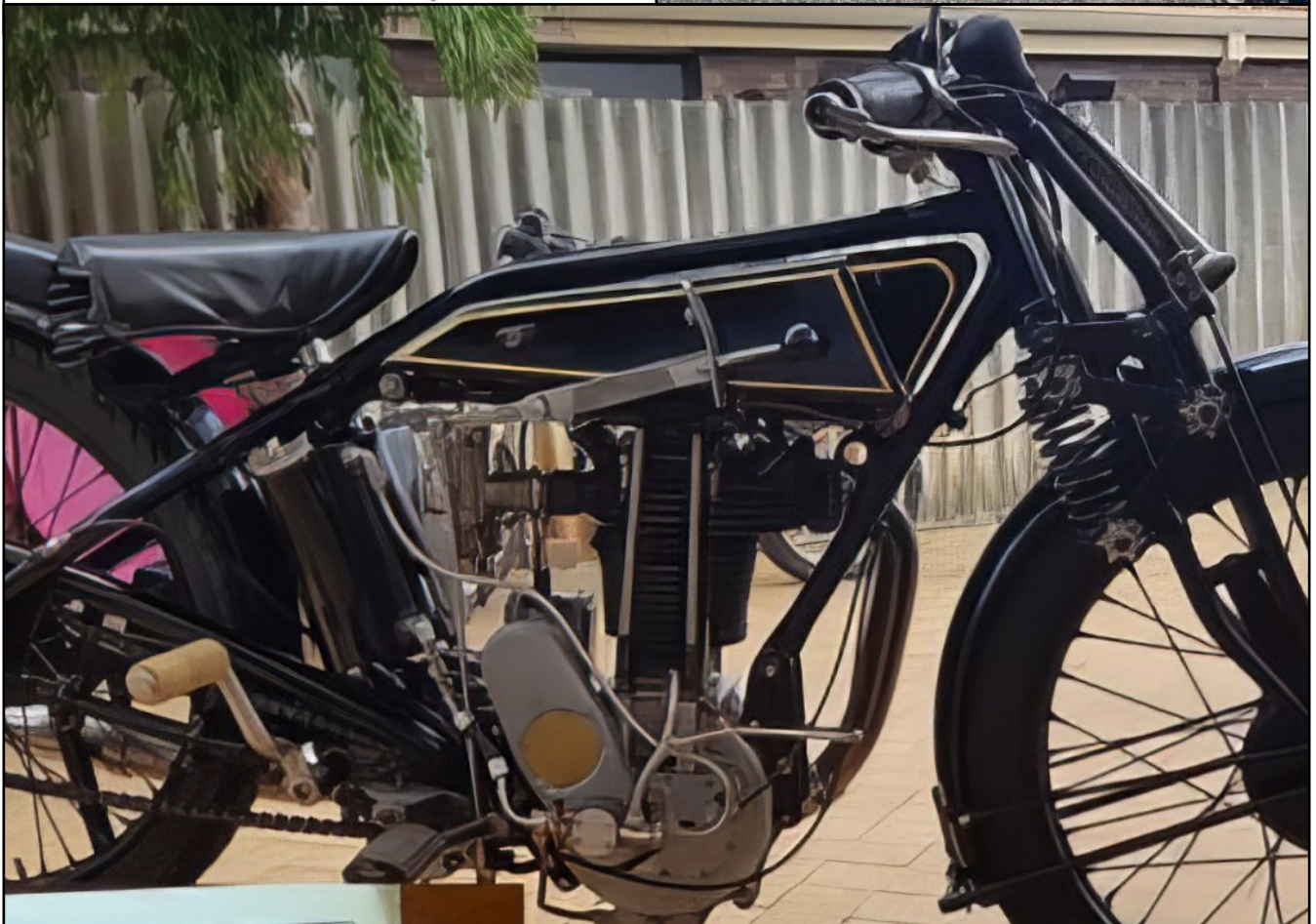
O.h.v. rocker details and cylinder head.
