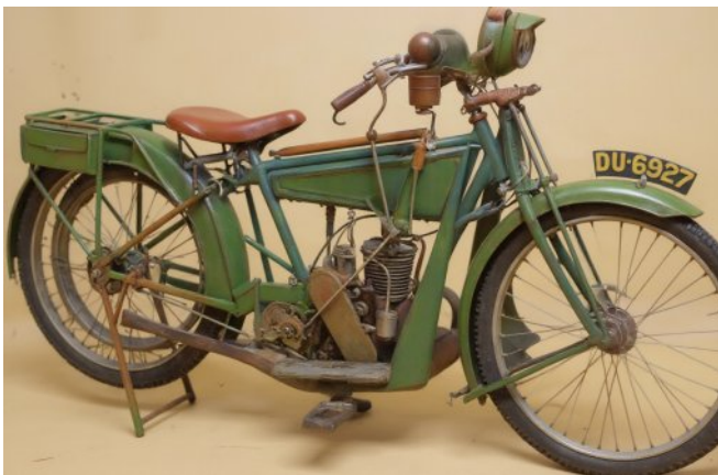
"A fine example of a British two-stroke design—the new Allon de Luxe, with spring frame and special mudguarding."
