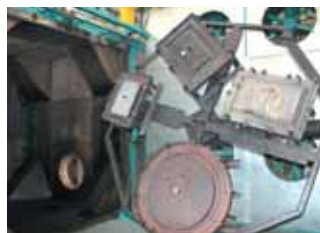
The mould is rotated in a specialised oven.
