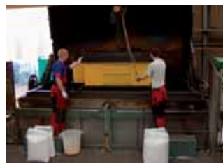
The powder transforms to liquid creating a plastic skin inside the mould.
