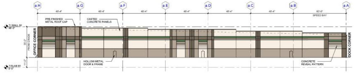
3 STREET FACING ELEVATION - BLDG. A SCALE: 3/16" = 1'-0"
