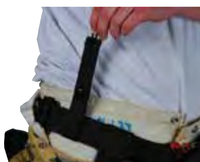
Harness keeper tab snaps around waist belt of harness.
