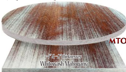
Whitewash - Oak veneer w/ engineered wood edge - stained, whitewashed, distressed then protective clear coat
