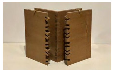
▲ Mizu-gumi ( nejire-gumi tsumi ) and Water joint (twisted tenon joint)
