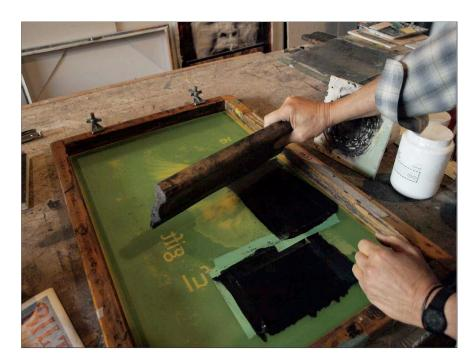
The photographic images and text were selected, then exposed onto screen printing frames. Ceramic enamels were applied through the screen mesh depositing the image onto glass.
