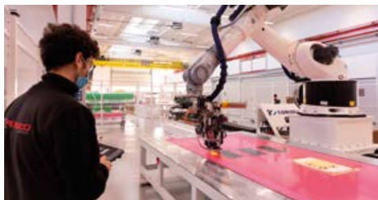
Automated tape laying robot 'Lola' at work.
