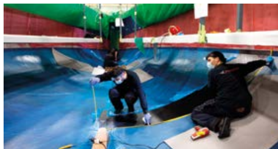
Prepreg carbon hull creation.
