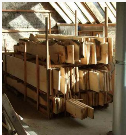
Vertical stacking of fresh sawn sycamore, Feb 2008. the stack was wrapped in card and warm air from the loft blown in until end of May.
