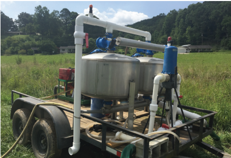
Example of a portable water treatment system used for irrigation
