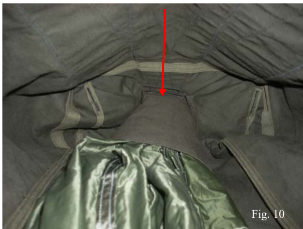
Fig. 10 Place the folded Apex Sleeve into the Deployment Bag and out of the far opening. (fig. 10)
