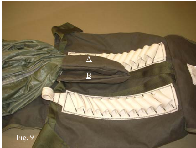
Fig. 9 Fold the Sleeve in half making sure to keep the canopy material (A) separated from the Apex lines (B). (fig. 9)
