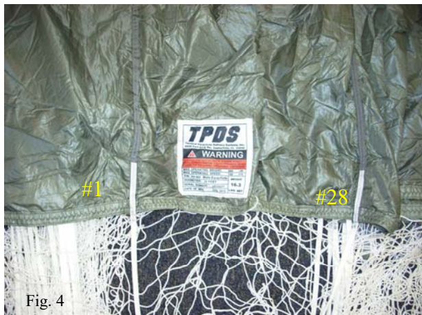
Pictured above is the top of the Main Parachute with data placard. (fig. #4)
