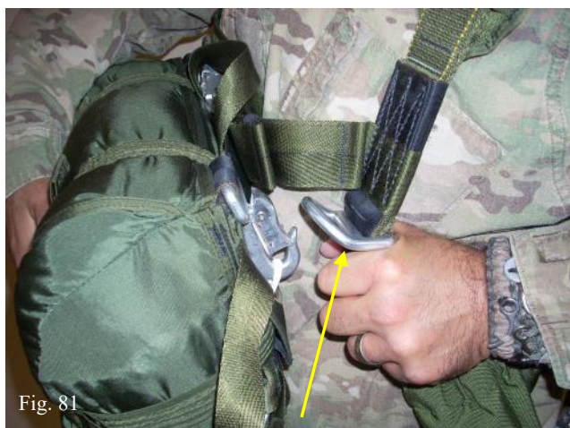
Hook up the Butterfly Snaps to the Main Lift "D" Rings and secure with the "safety pin". (fig. # 81)
