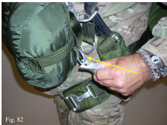
Hook up the Alligator Clips of the Reserve Side Connectors to the Reserve Container Rings and adjust snug. (fig. # 82)
