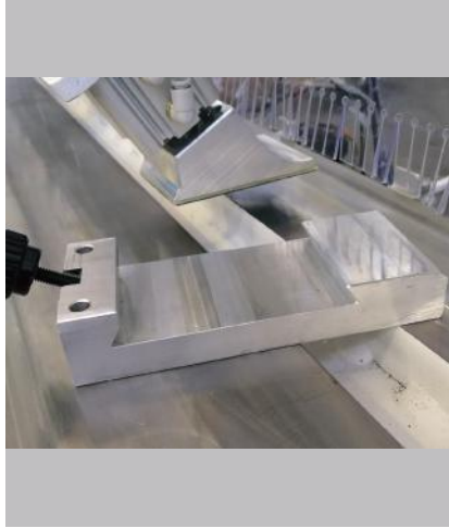
Clamp pad extension for pressing pieces minimum width 40 mm.
