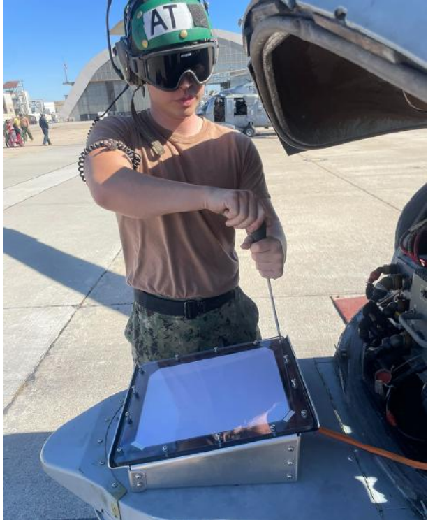
An AT secures the plexiglass over the Starlink mini antenna mounted on the nose of HSC-23's MH-60S helicopter.
