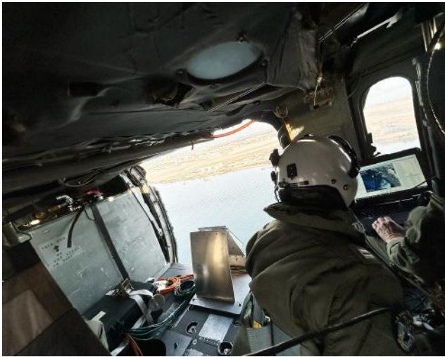
Taken inside the cabin of a MH-60S. The DESM Antenna is mounted on the side of the port cabin door, and the aircrewman is looking at the geospatial display of surface geolocations being provided by the equipment.
