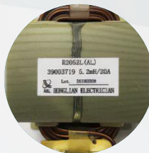
Reactor for Single-Tube BOOST-PFC
