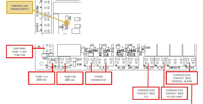
Closes when the unit breaks down Can be applied in a domotic system to indicate a failure
