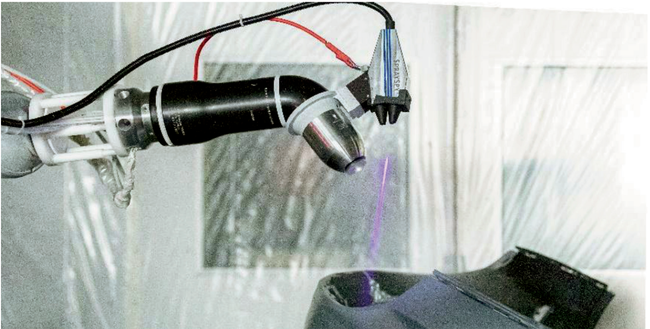
Fig. 2: Online Spray measurement while painting bumper
