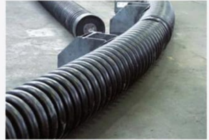
Bending of Durapipes R/D = 30
