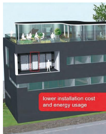
Complex AHU installations, which may include a boiler and chiller plant, can be replaced by an AHU with integrated reversible heat pump
