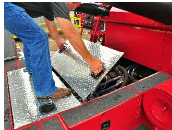
Lightweight Deck Lids Provide Easy Access to Drivetrain & Hydraulics
