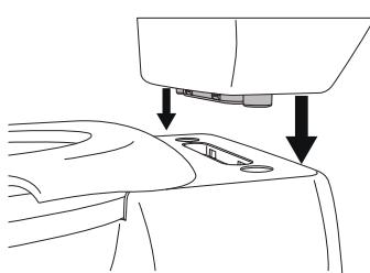
**2** Insert the tank into the holes on the base, push firmly until all 4 snaps lock in.
