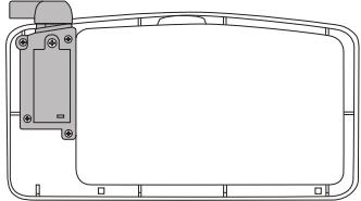
Locate battery compartment attached to flush handle in tank lid.
