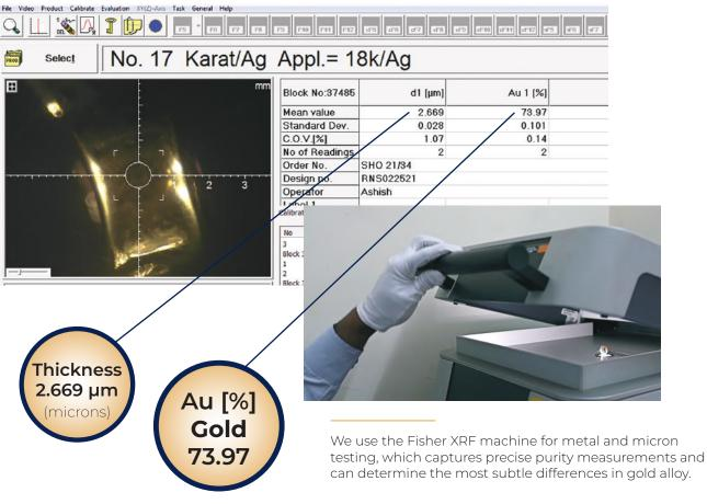
The certified standard for vermeil gold is 2.5 microns thick. Our test results exceed the standard at 2.669 microns, and show almost 74% for gold purity.
