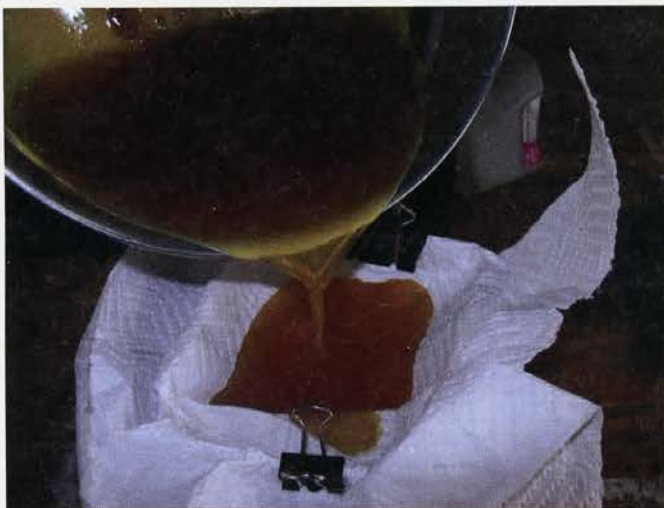
Melt the wax again and use a filter to remove impurities. I like sweatshirt material, but paper towels work too.
