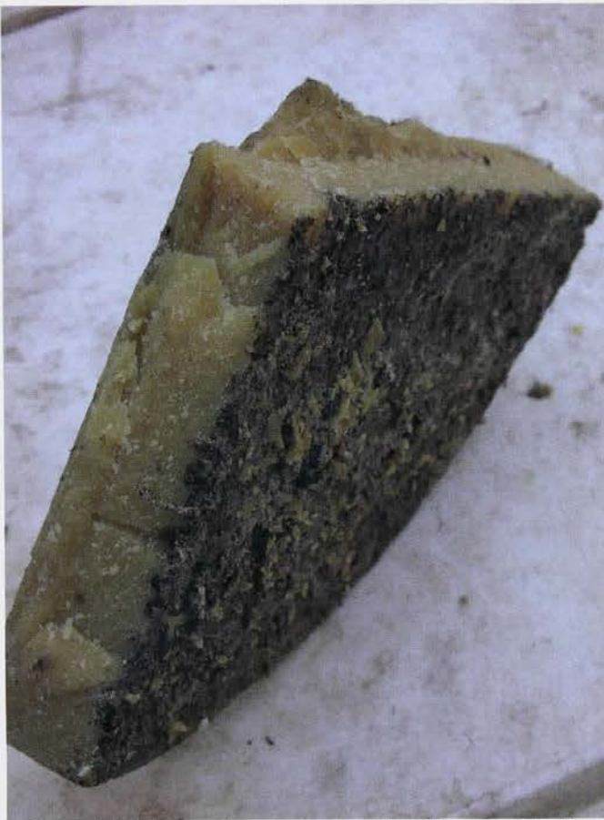
Dirt and debris that clings to the wax should be scraped off before remelting.
