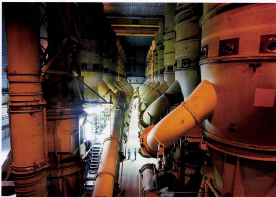
▲ Gas diffusion machinery in southern France used to enrich uranium for use in nuclear reactors.
