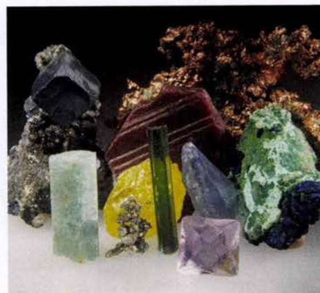
▲ Assorted minerals, including elements such as sulfur and silver, and compounds such as \text{Al}_2\text{O}_3 (sapphire) and \text{CaF}_2 (fluorite). Most minerals are impure and exist as mixtures of different elements and compounds.
