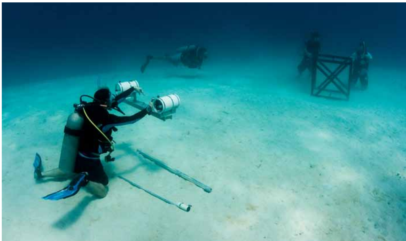
University volunteers from the US help Operation Wallacea scientist calibrate a stereo-video system used to calculate the biomass of fish present on coral reef sites in Honduras in 2012.
