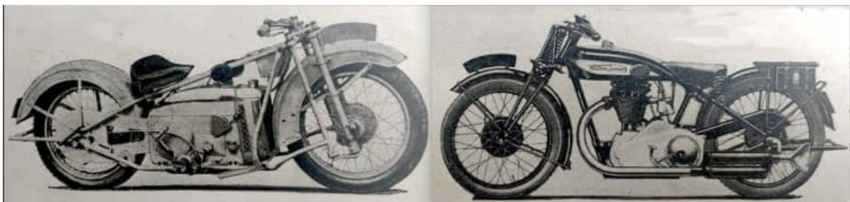
L-R: "The water-cooled OEC-Tinkler has the engine and gear box combined in one unit. The new 348cc ohc Norton 'Junior'."
