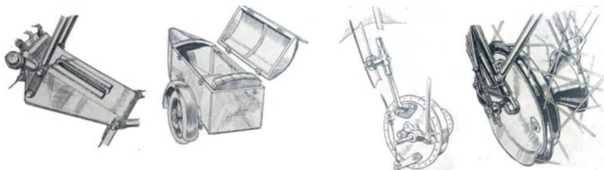
L-R: "Combined oil tank and gear box bracket on the 198cc OK-Supreme. A combined dual-purpose Baker sidecarrier finished in black leather cloth and white piping. Front brake anchorage on Indian models; the sliding members can be lubricated by grease gun. Front brake
