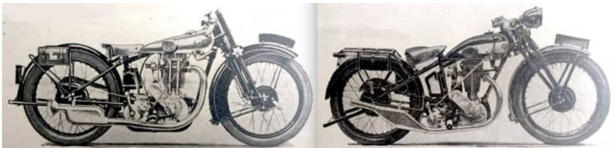
L-R: "Graceful lines characterise the 'Special sports' Grindlay-Peerless. It is fitted with a 490cc twin-port JAP engine and Castle forks. Important modifications to the 346cc ohv Levis give it the appearance of an entirely new type."
