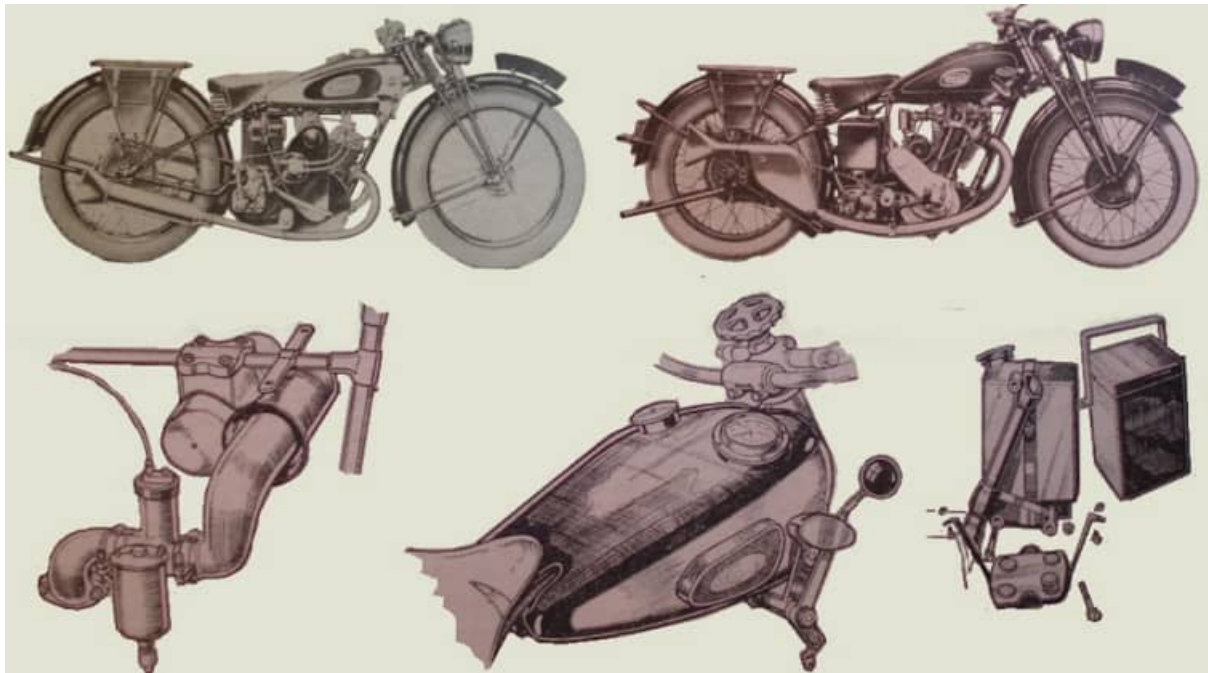
L-R: "The 'K' Royal De Luxe model in its latest form. (Right) A smart thoroughbred—the 496cc model 'S' four-stroke. The air silencer on the two-stroke models is now tucked away beneath the tank. The new and more graceful tank. The oil tank and battery box on the Montlhéry model are carried on platforms attached to a lug on the seat tube."
