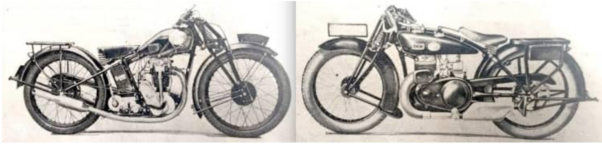
L-R: "The neat 349cc ohc Humber engine is now housed in a particularly sturdy cradle frame. Air-cooled 292cc two-stroke DKW."
