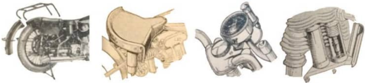
L-R: "How the BS carrier and mudguard flap may be detached, leaving the tool bags in situ. The enclosed-spring Brough-Superior-Lycette saddle, with Sorbo back edge. On all models a speedometer lamp is fitted to an extension of the instrument bracket. The valve covers on the SS80 are split vertically, quickly detachable and oil tight."
