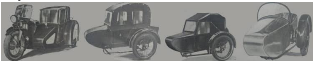
L-R: “An innovation—the Ascot-Pullin pressed steel sidecar in which the body forms the chassis. An example of modern sidecar practice is the Milford ‘Saloon’. The tandem two-seater Watsonian is suitable for any weather. An attractive semi-sports sidecar—the Model 7 Swallow.”
