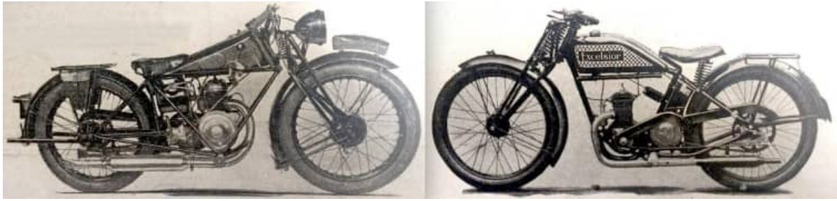
L-R: "The 172cc Villiers-engined Francis-Barnett is greatly improved by the provision of a neat saddle tank. 147cc Excelsior—a sturdy ultra-lightweight."
