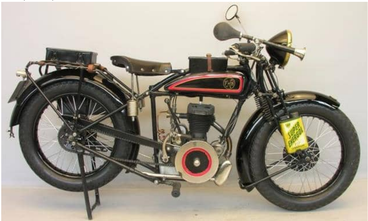
Two french army officers, Captain Bruneteau and Lieutenant-Colonel Gimie, and a Belgian mechanic, Joseph Weerens, rode 350cc sidevalve FN M70s across the Sahara. The bikes, fitted with larger tanks and saddlebags, covered 8,800km, including 6,300km of desert; the M70, marketed as the Sahara, was FN's most successful model of the inter-war period. The external flywheel of the early models was coloured red, inspiring the memorable nickname 'Moulin Rouge' (red windmill).
