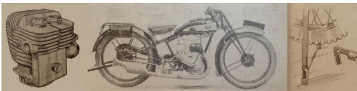
L-R: "Enclosed valve mechanism on the 250cc side-valve model. The cover is easily detachable by the removal of a milled nut. The new 250cc side-valve four-stroke Levis. A 'false foot' on the Levis stand for use in gutters."
