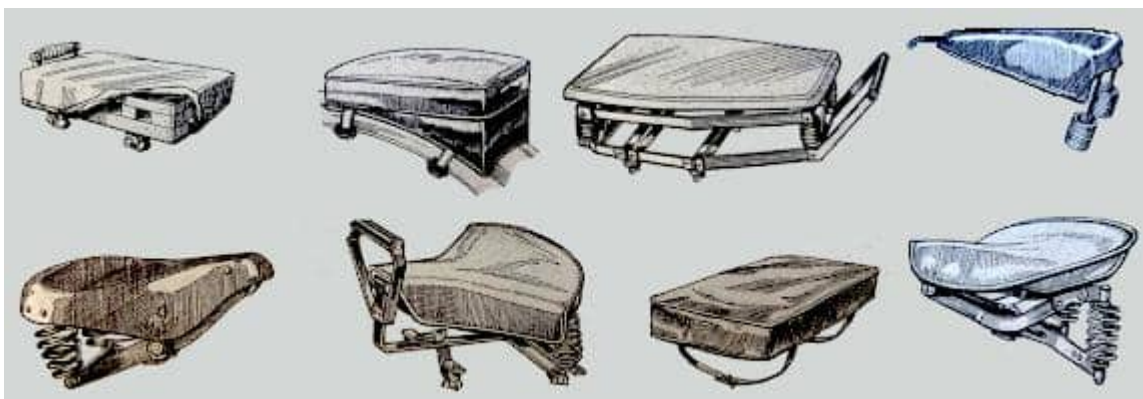
Top row L-R: “Sorbo pillion seat with sponge-rubber padding. P&H pillion seat for carrierless mounts. Leatheries ‘Safastri’ pillion seat, shaped for astride riding. Gough frameless saddle for direct fixing.” Bottom row L-R: “The Dunlop rubber-topped waterproof saddle. Saddle-type Leatheries pillion seat. The latest Brooks pillion air cushion. Brooks pan-seat saddle.”
