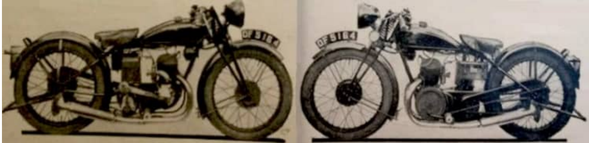
"The new Velocette two-stroke with foot gear change and coil ignition."
