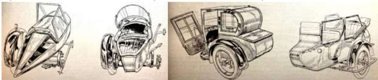
L-R: "The Watsonian 'Kwikfit' sidecar is quickly detachable and has a 'prop wheel'. A luxurious Brough Superior sidecar has a floating sidecar wheel and rear connection. A car on one wheel! The Tornado sunshine saloon. A family sidecar in full sail—the two-seater AJS."
