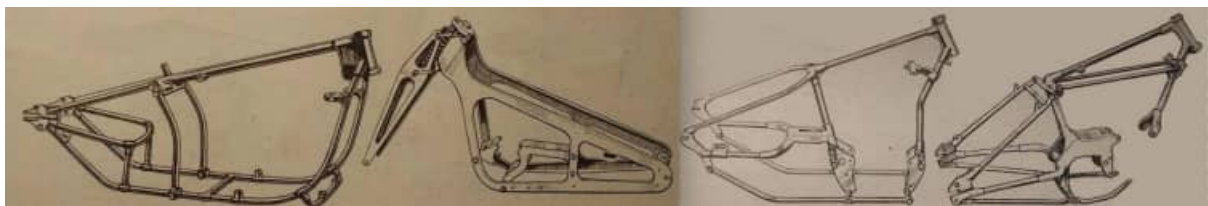
L-R: "Frame of the experimental Brough Superior four-cylinder machine. Coventry-Eagle lightweight pressed-steel frame. Coventry-Eagle frame and torque tubes of the 490cc model. Matchless frame, in which bent tubes are avoided."
