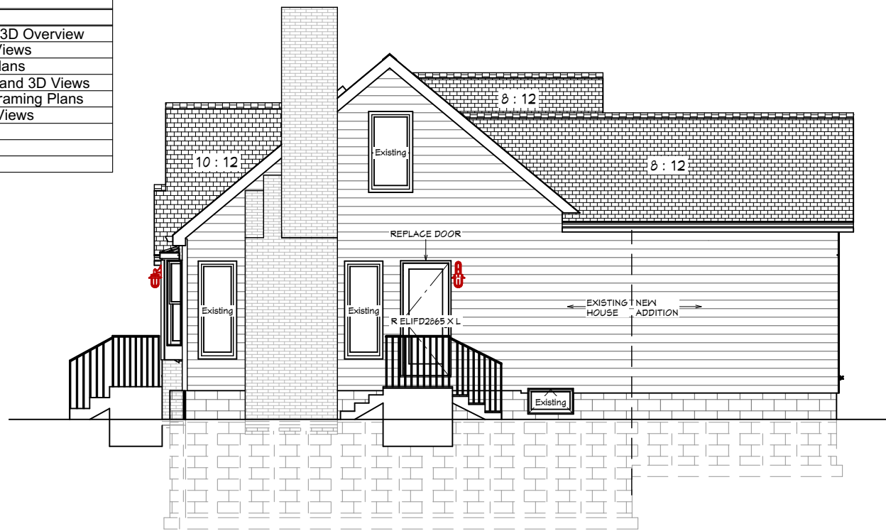
B NORTH ELEVATION 1/8 in = 1 ft
