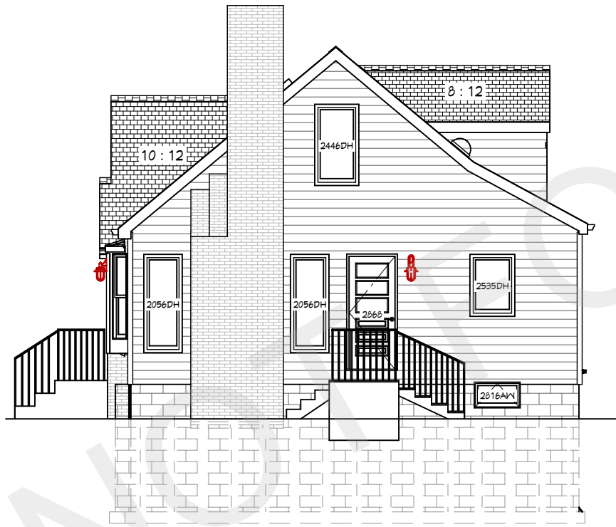
B NORTH ELEVATION 1/8 in = 1 ft
