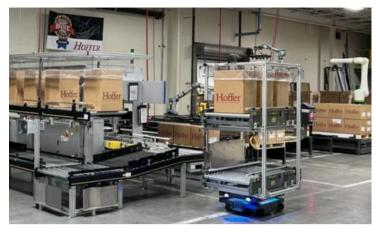
Hoffer Plastics has significantly boosted efficiency and safety through the implementation of autonomous mobile robots (AMRs) and cobots. These technologies enhance part inspection, filling, palletizing, and transport, resulting in over 55,000 hours of saved manual labor. Additionally, AMRs have reduced annual lifting by up to 2 million pounds, improving employee safety. Ongoing investments in automation support both operational improvements and consistent product quality. MORE
