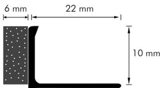
**JUNTA CON ESPUMA 10mm**
