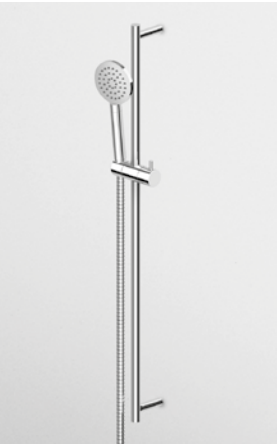
COMPLETE SLIDE RAIL Complete slide rail with adjustable bracket, length 29 5/8", handshower Z94300, 59" flexible hose.
