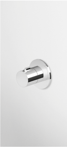
2 WAY DIVERTER 2 way diverter without water on/off function, 1/2" outlets. To be combined with a built-in single lever shower mixer.
