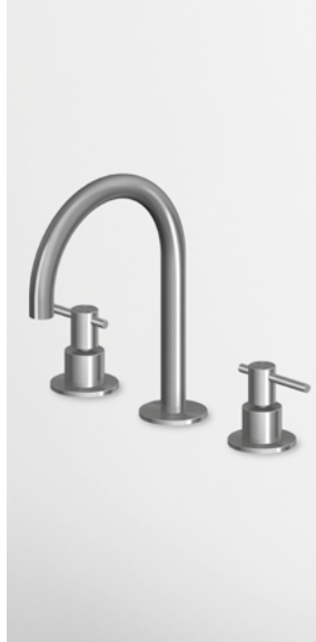
BASIN 3 hole basin mixer with aerator, flexible hoses, without pop-up waste. Spout projection 5 7/8". Water flow restricted to 1,2 GPM
