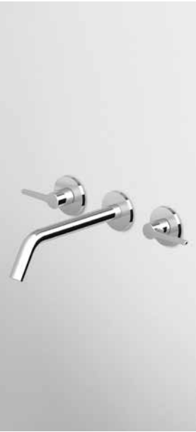
BASIN 3 hole built-in basin mixer with aerator. Spout projection 8 1/2". Water flow restricted to 1,2 GPM
