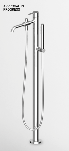
BATH Free standing single lever bath mixer with diverter and handshower Z94727, 59" flexible hose. Spout projection 9 13/16". Water flow restricted to 2,4 GPM (handshower).
