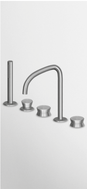
BATH 5 hole bath-mixer, spout with diverter, pull out shower Z94249.1900X, 59" flexible hose. Spout projection 8 3/4". Water flow restricted to 2,4 GPM (handshower).
