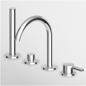
BATH 4 hole bathtub single lever mixer, swivel spout or lockable during installation, pull out shower Z94177.1900, 59" flexible hose. Spout projection 7". Water flow restricted to 2,4 GPM (handshower).
