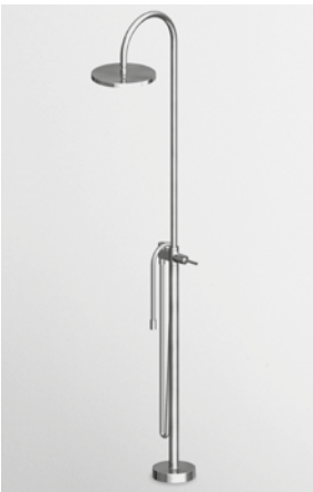
SHOWER COLUMN Stainless steel free standing shower column for outdoor use, single lever joystick mixer, rain shower head Ø 11 3/4", foot washer with elastomer hose.
