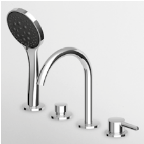
BATH 4 hole bathtub single lever mixer, swivel spout or lockable during installation, pull out shower Z94746, 59" flexible hose. Spout projection 7". Water flow restricted to 2,4 GPM (handshower).
