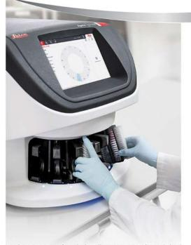
Aperio GT 450 open face design allows you to continuously load racks while scanning is in progress to maximize productivity.
