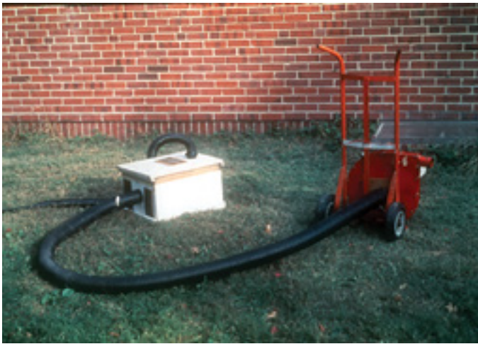
The 1976 model vacuum device. The smaller vacuum line entering on the top empties into a screened package bee cage.
