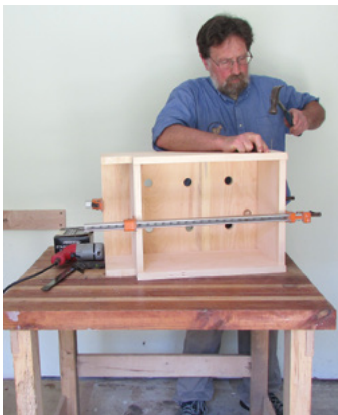
Fastening ends to sides.
