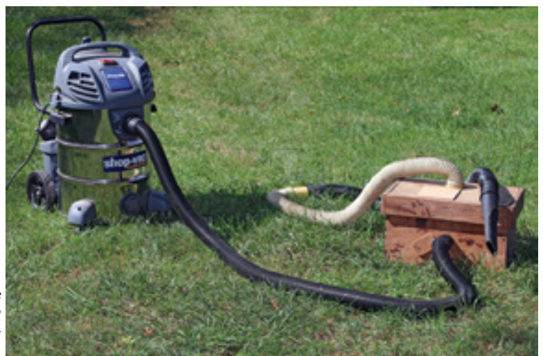
Shop vac modified to provide vacuum to the trap box.
