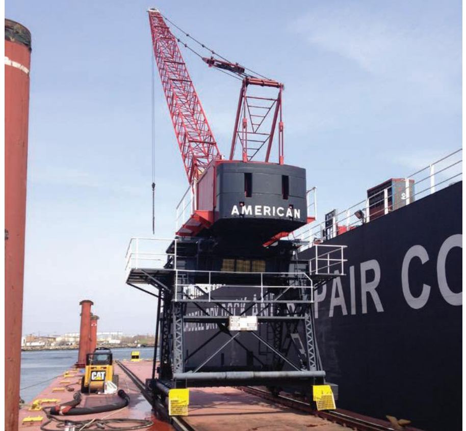
Fig. 4. Portal cranes can be reconfigured for heavy lifts.
