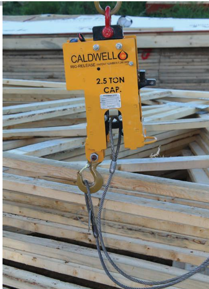
This hook is unable to release the load until it has been set.
