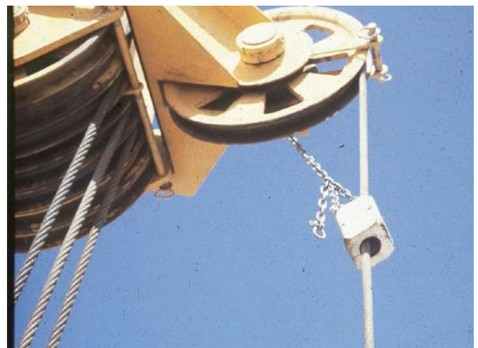
Fig. 2: If a block raises the bobweight, the hoist will stop.
