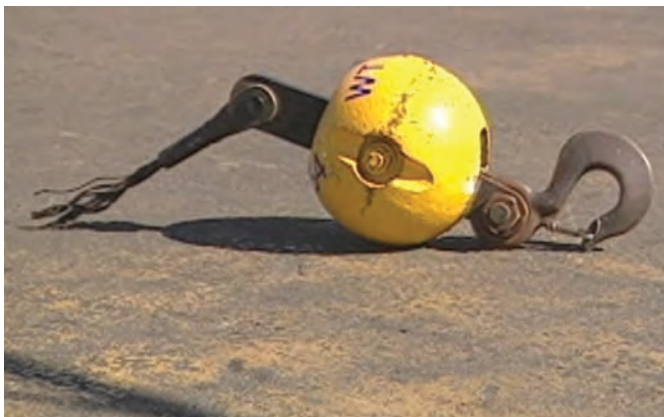
Fig. 1 The rope parted when the hydraulic boom was extended, and a limit switch failed.
