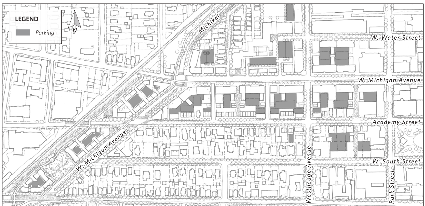
FIGURE 97: Use of Parking Courts in Interior Blocks Instead of parking lots along streets, which impair the public realm, the proposal provides space at the interior of the blocks for parking courts for larger building types, or garages for smaller residences. Consider an overall, citywide parking strategy to distribute parking among these blocks.
