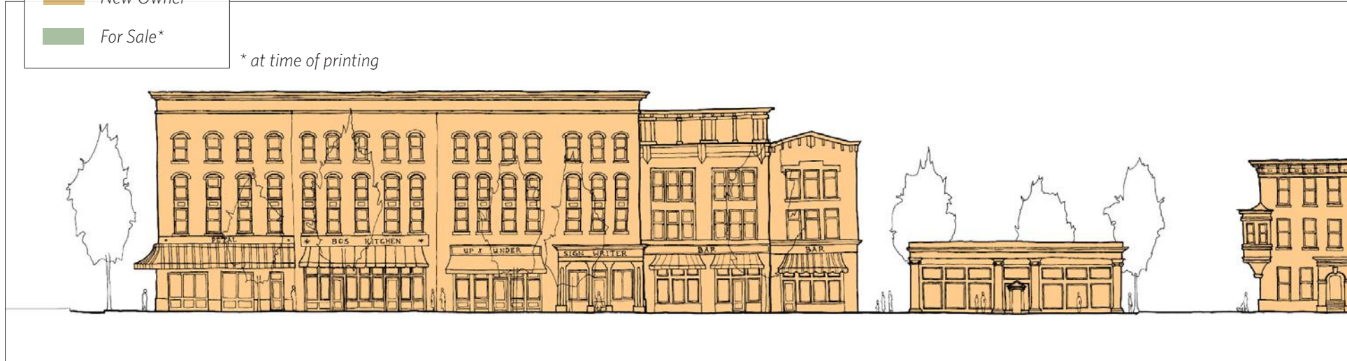
FIGURE 90: Building Divisions by Property Ownership along W. Michigan Avenue, Facing South The orange, yellow, and green overlays indicate three different property owners with different property widths. It is possible to achieve a consistent rhythm along the street by strategically dividing facades within aggregated parcels.
