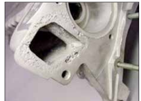
Electrolysis damage due to poor cooling system maintenance
