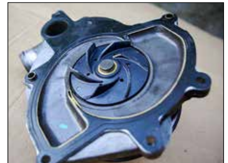
Water pump impeller failure example
