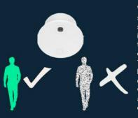
When occupancy is detected, the heating system automatically turns on. Here are some additional points that you could include: The system can be programmed to turn on when occupancy is detected during certain times of the day or in specific rooms. This feature helps to save energy by only heating the rooms that are in use. The system can also be configured to turn off the heating when no occupancy is detected for a certain amount of time, further reducing energy consumption.
