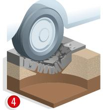
When vehicles drive over this cavity, the pavement surface cracks and falls into the hollow space, leading to the birth of another pothole.
