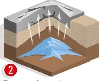
The moisture freezes when temperatures drop, causing the ground to expand and push the pavement up.
