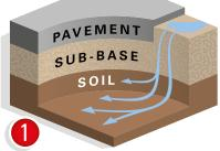
Potholes begin after snow or rain seeps into the soil below the road surface.
