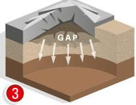
As temperatures rise, the ground returns to normal level but the pavement often remains raised. This creates a gap between the pavement and the ground below it.
