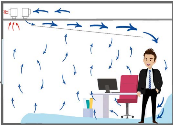
When a jet of air hits the wall (Left) or a jet travelling from the opposite direction (Right) it descends into the occupied zone.
